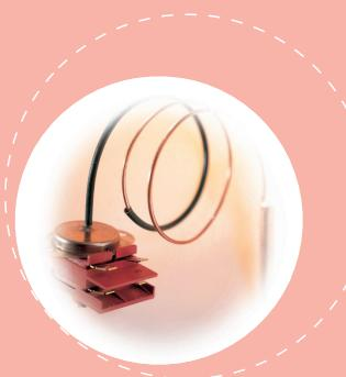
The L Series, L7, LM7 and LM8, is a family of fixed setting temperature limit controls whose design is fail-safe. The L7 is auto reset, whilst LM7 and LM8 are manual reset. The operating temperatures are factory set and non-adjustable by the customer. Settings are available between 50 and 160°C with capillary lengths from 450 - 2000 mm (1000 mm standard). The L7/LM7 are SPST (single pole single throw) and LM8 is DPST (double pole single throw).
